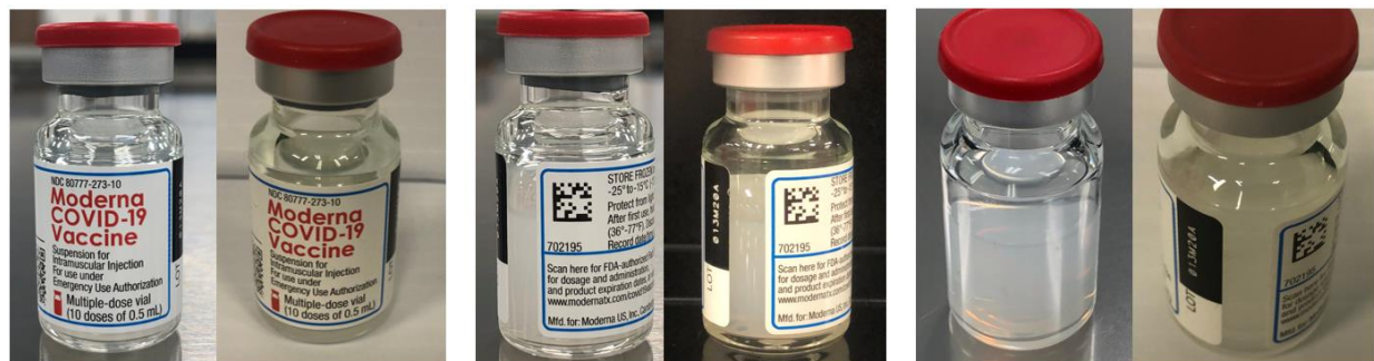
1 Typical range of coloration of Cyclic Olefin Polymer (COP) vials, SiO2 Materials Science, 2020
